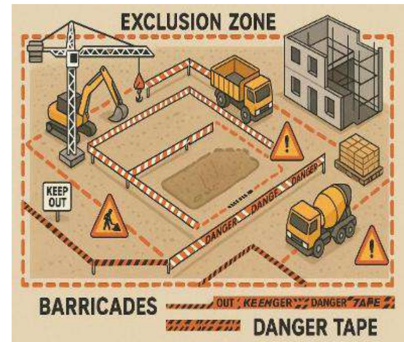
Figure 9: Typical exclusion zone signalling
